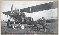
crew and mechanics see to their various tasks. The cowl (MS) behind the engine has been removed while "something" is checked.
